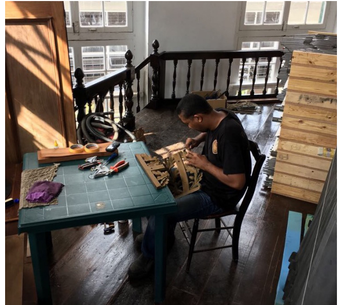
Rafael van Ommeren carries out restoration work on parts of the organ in the Maarten Lutherkerk in Paramaribo (photo: Peter van Rumpt, organ restorer).
